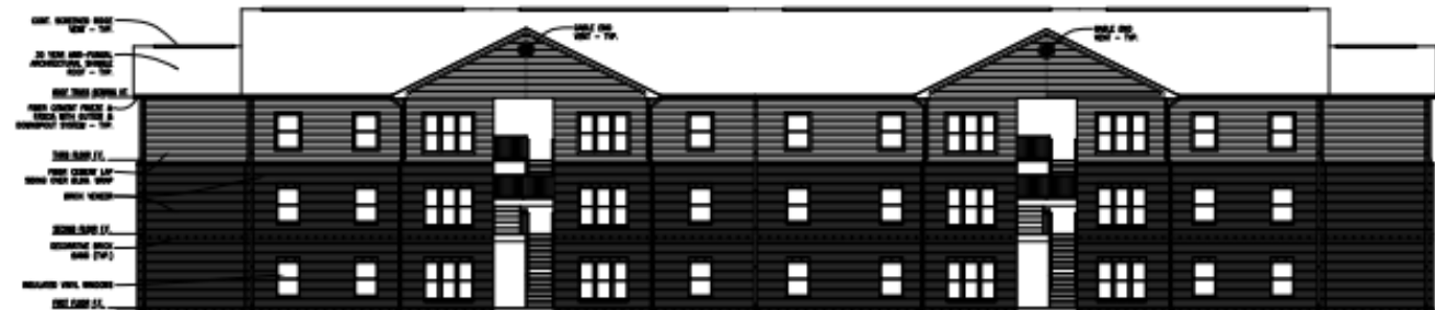
BUILDING TYPE A BUILDINGS 1 & 4 FRONT AND REAR ELEVATION SCALE: 1/8"=1'-0"
