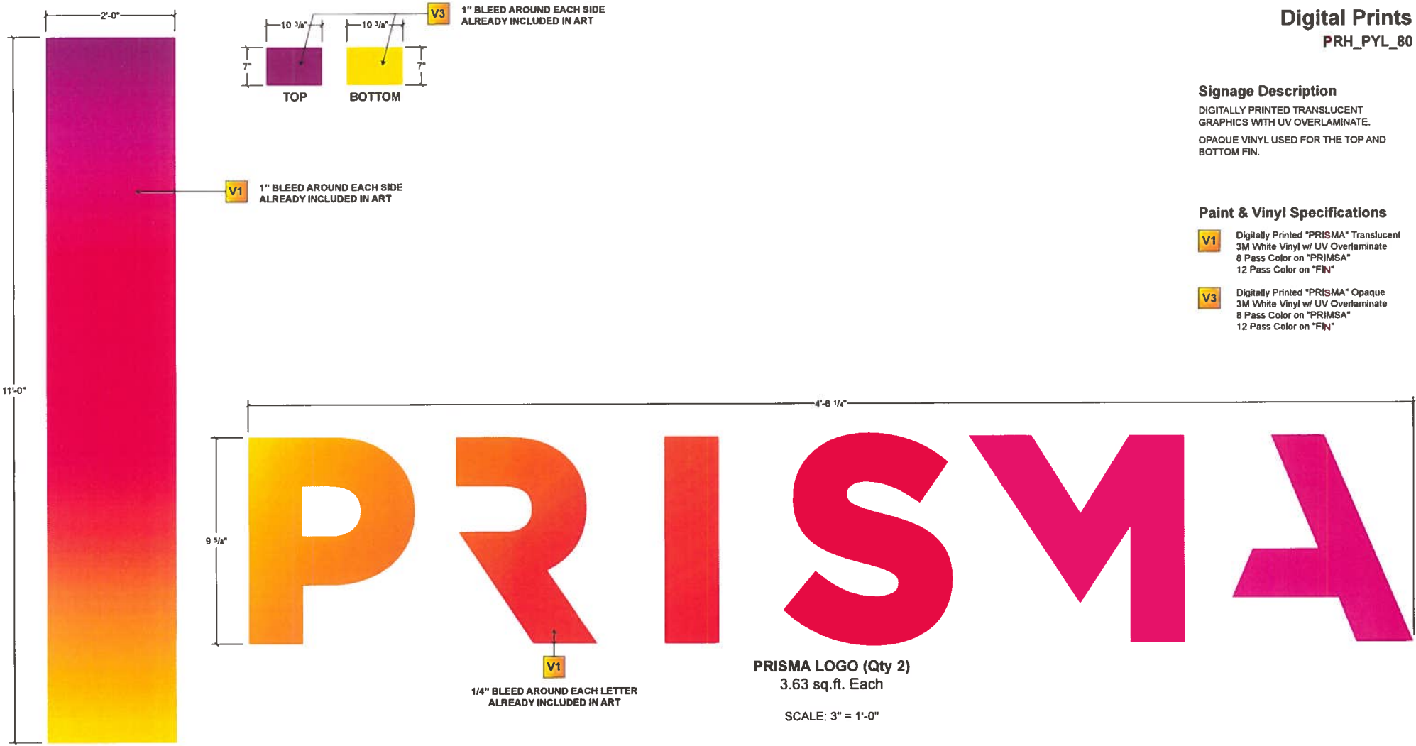
FRONT AND SIDES PRISMA FIN (Qty 1) 23.01 sq.ft SCALE: 3/4" = 1'-0"
