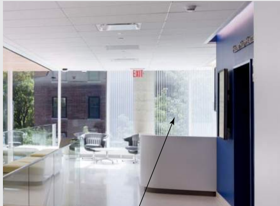
Glass Type II: CW with Vertical Line Ceramic Frit Pattern
