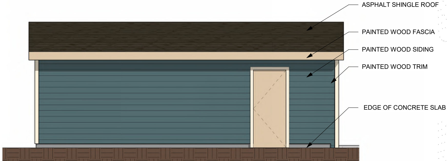
2 GARAGE ELEVATION - WEST 1/4" = 1'-0"
