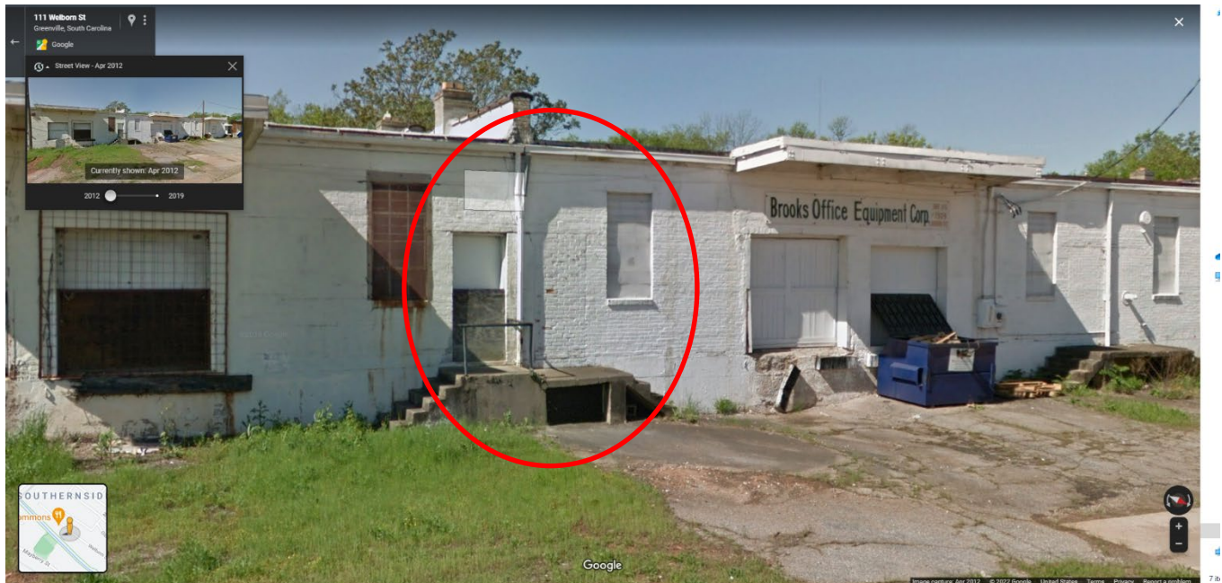
Figure 1: Google Street View imagery from 2012 showing the subject property with doorway circled. At the time, the doorway was bricked in, although the remnants of the original opening are visible.
