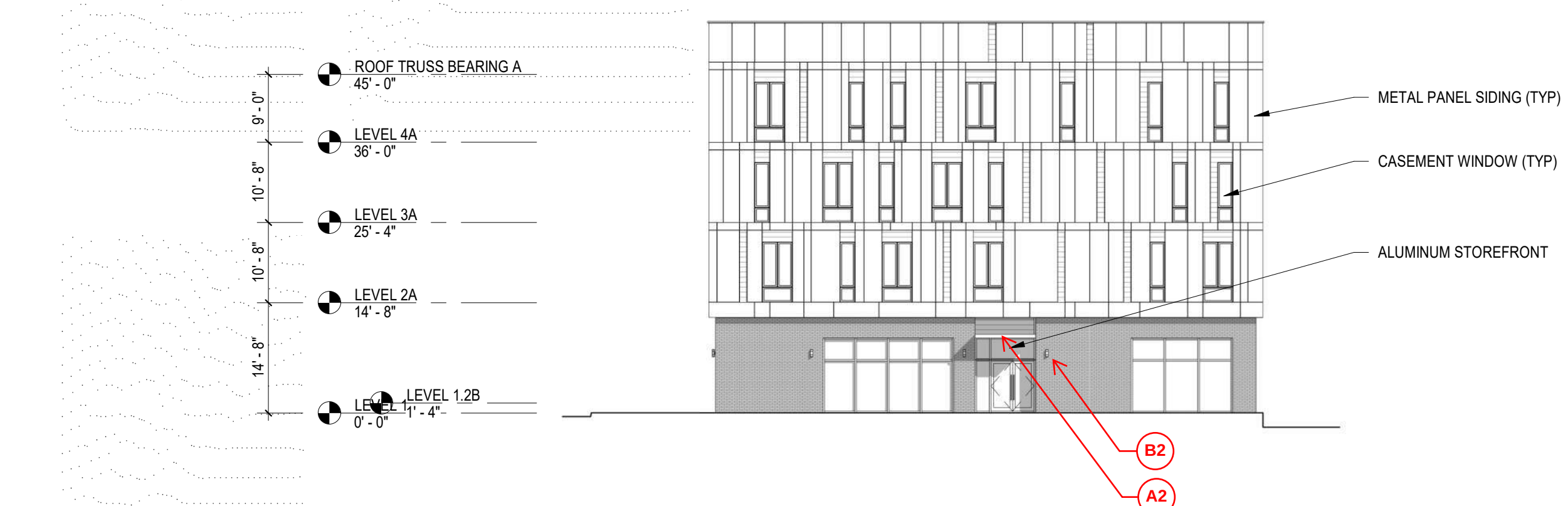
A4 PARTIAL WEST ELEVATION - BUILDING A A2.01 1/16" = 1'-0"
