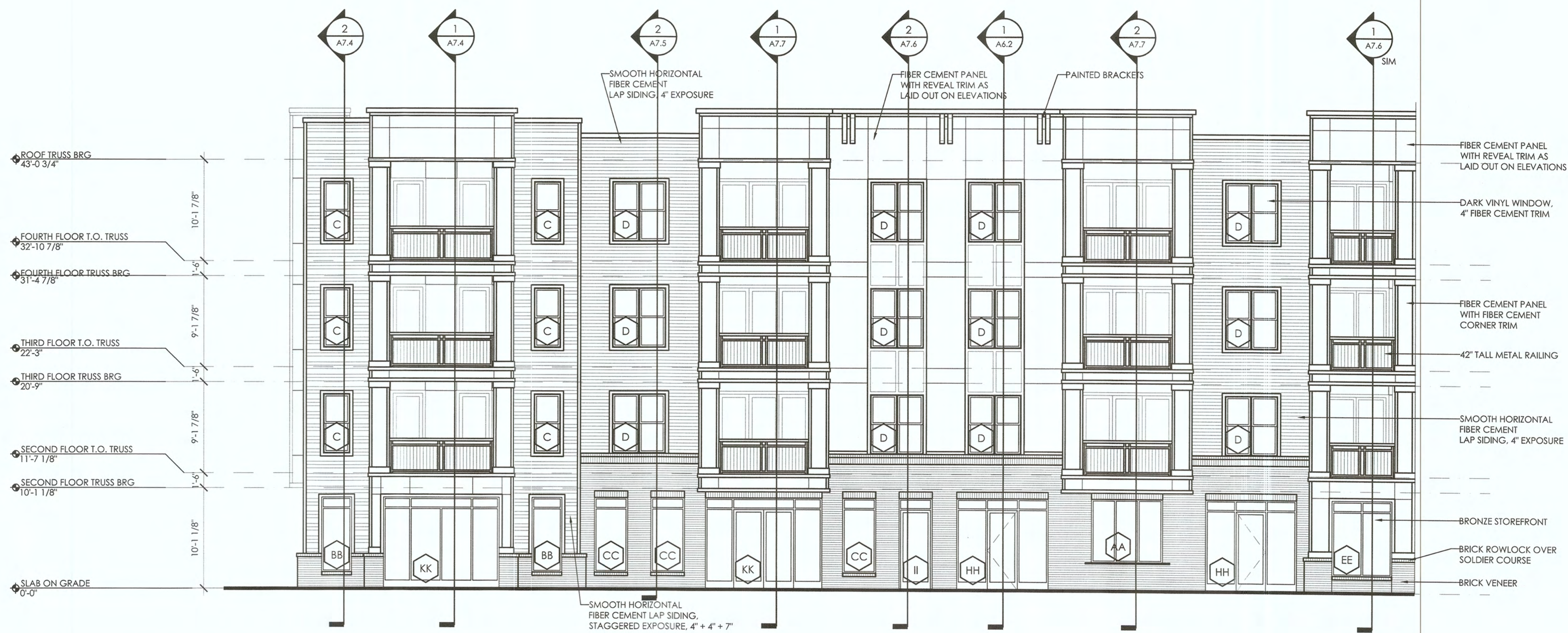
1 BUILDING ONE COURTYARD ELEVATION AT FITNESS 1/8" = 1'-0"
