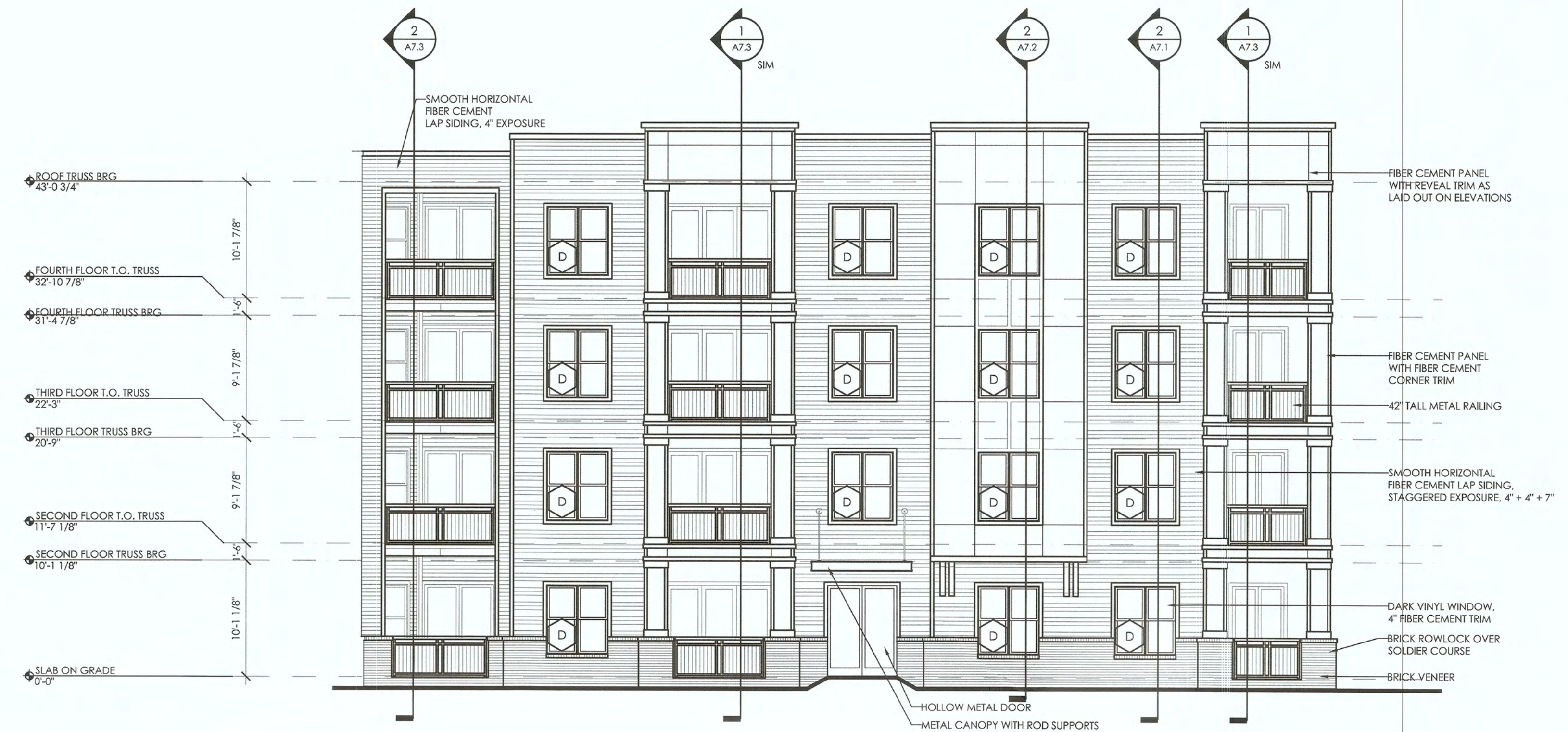
2 BUILDING ONE COURTYARD ELEVATION AT BUILDING ENTRANCE 1/8" = 1'-0"
