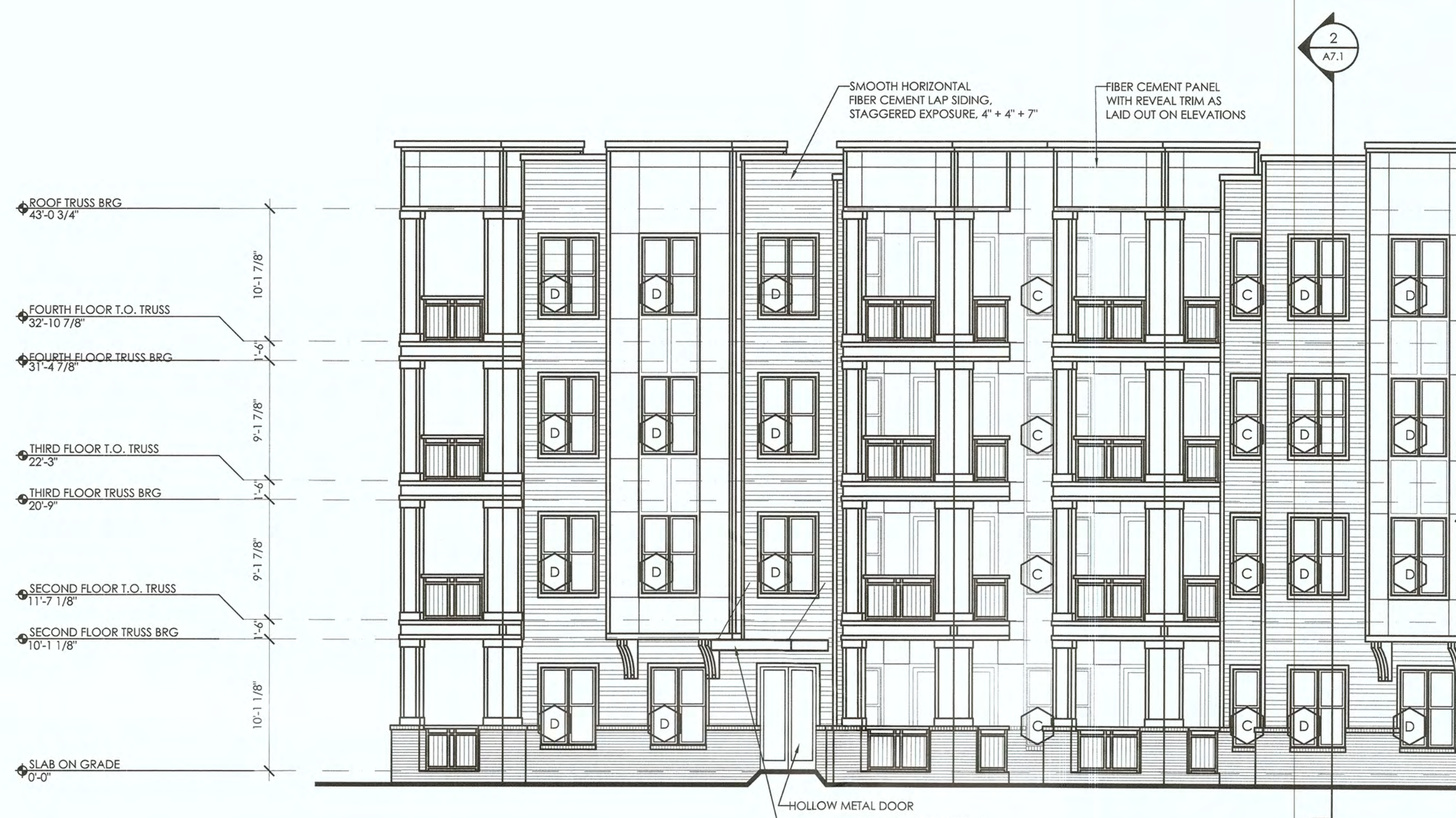
2 BUILDING ONE FRONT ELEVATION - CONT. 1/8" = 1'-0"
