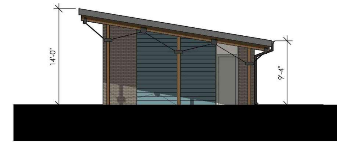
MAINT. GARAGE - WEST ELEVATION SCALE: 1/8" = 1'-0"
