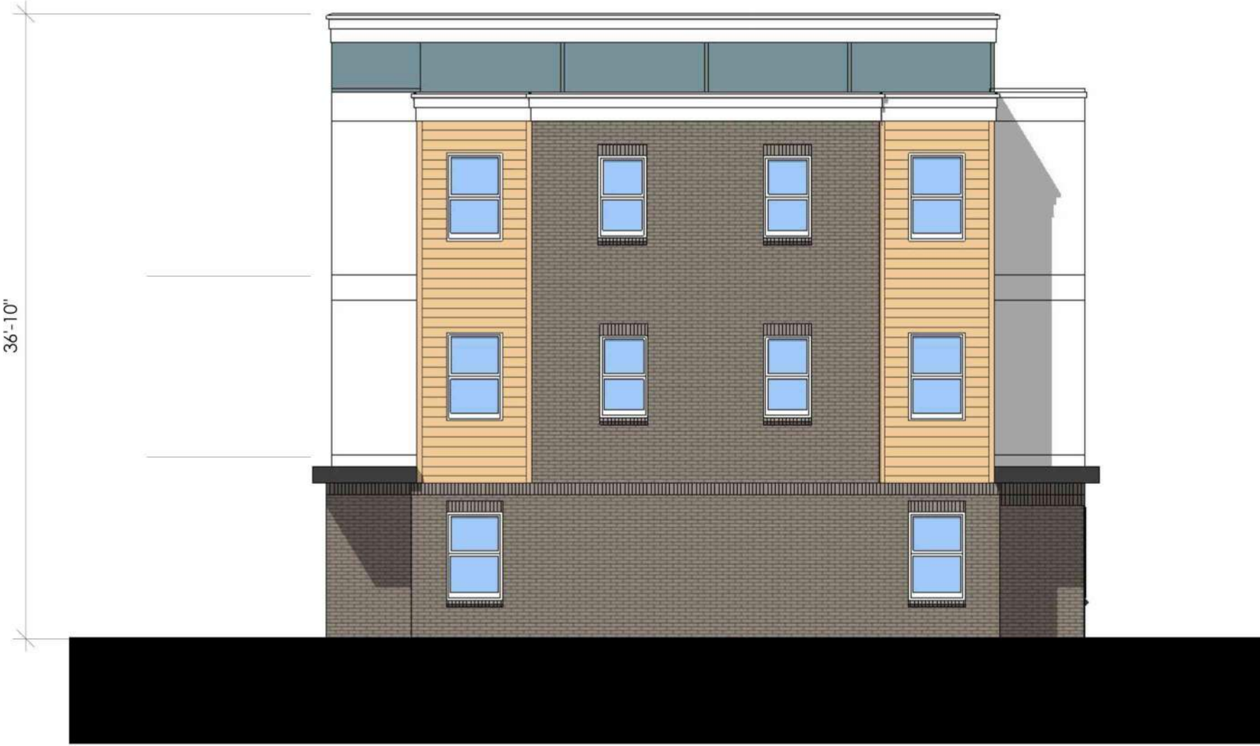
BUILDING TH - SOUTH ELEVATION SCALE: 1/8" = 1'-0" 3-STORIES / 6 UNITS
