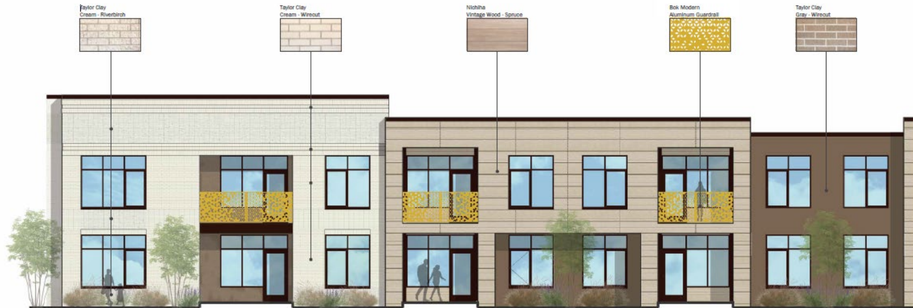
02 ENLARGED ELEVATION: Pendleton Street Elevation - Partial 1/4" = 1'-0"
