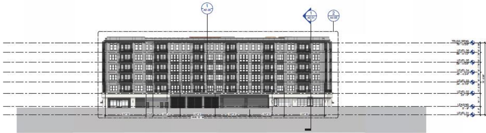
2 OVERALL ELEVATION - WEST (ALLEY) SCALE: 1/8" = 1'-0"
