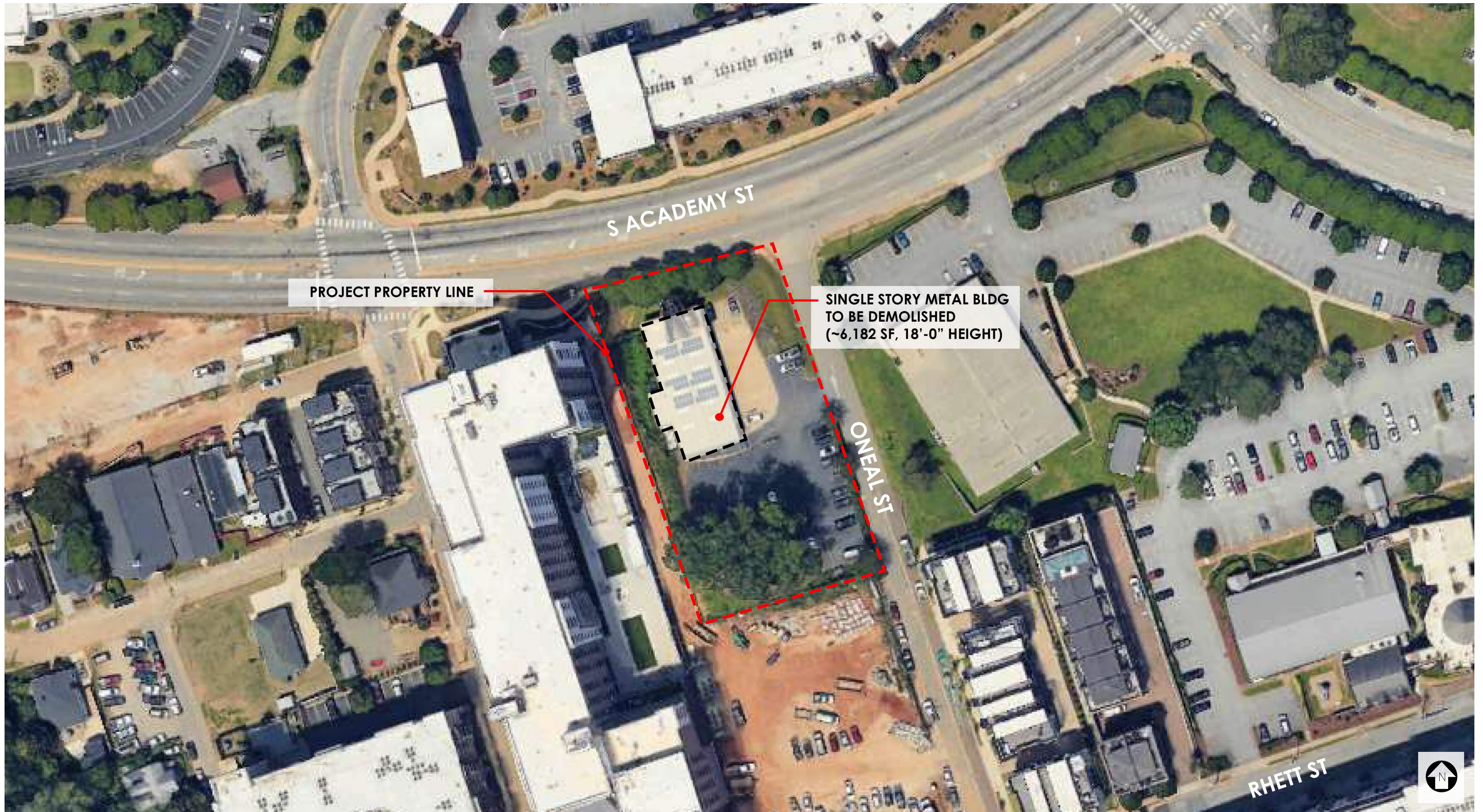
SITE PLAN - EXISTING CONDITION
