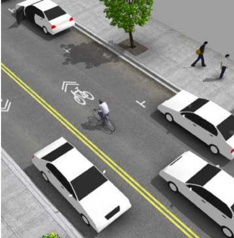
Level 1 Shared Lane
