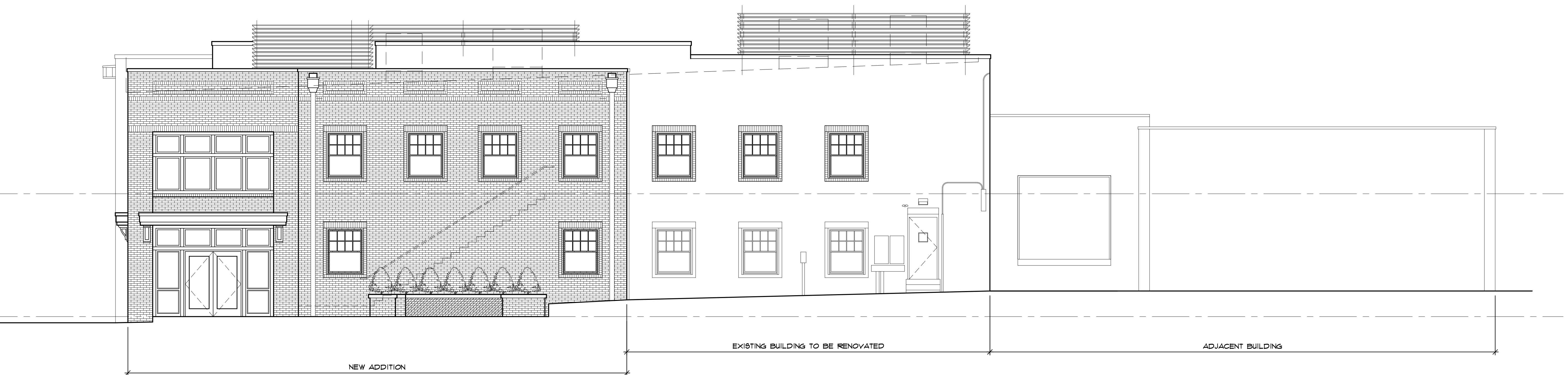
2 WEST EXTERIOR ELEVATION W/ ADJACENT BUILDING SCALE: 3/16" = 1'-0"
