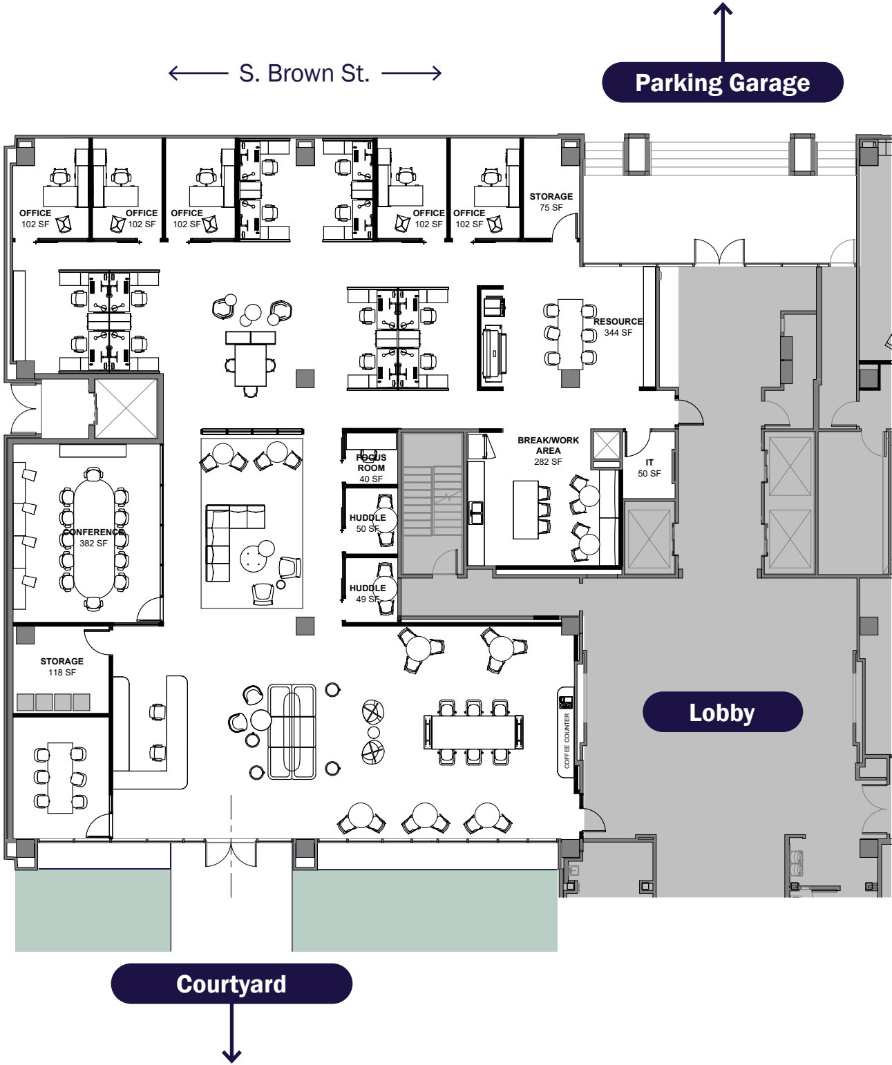
1st Floor - Proposed Plan 1/16" = 1'-0"
