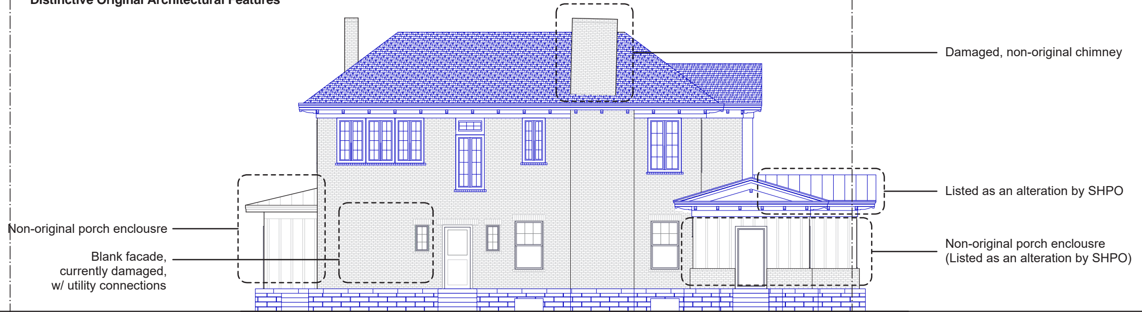
Overview of Existing Distinctive Original Architectural Features
