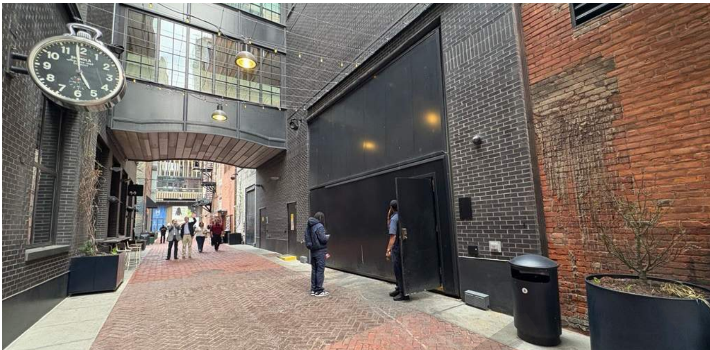
Placing trash is clustered and tucked out of the pedestrian passageway with a solid door that blends with the building and pedestrian passageway design.
