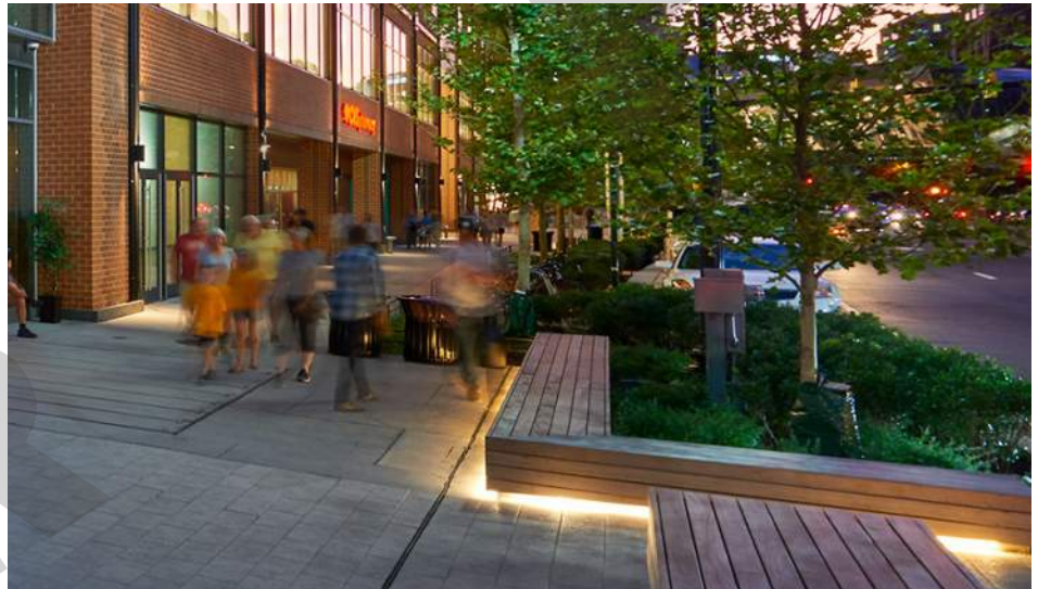
On-street parking in high retail area. There is a clearance zone for passengers to exit parked cars, a planting zone, and a clear path for pedestrians.
