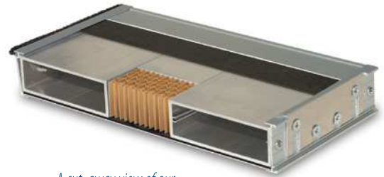
A cut-away view of our Series 100BE reveals the 5-ply construction which includes full perimeter aluminum frame, high compression honeycomb core, and aluminum facing with tempered organic backing (on both exterior and interior door surfaces).
