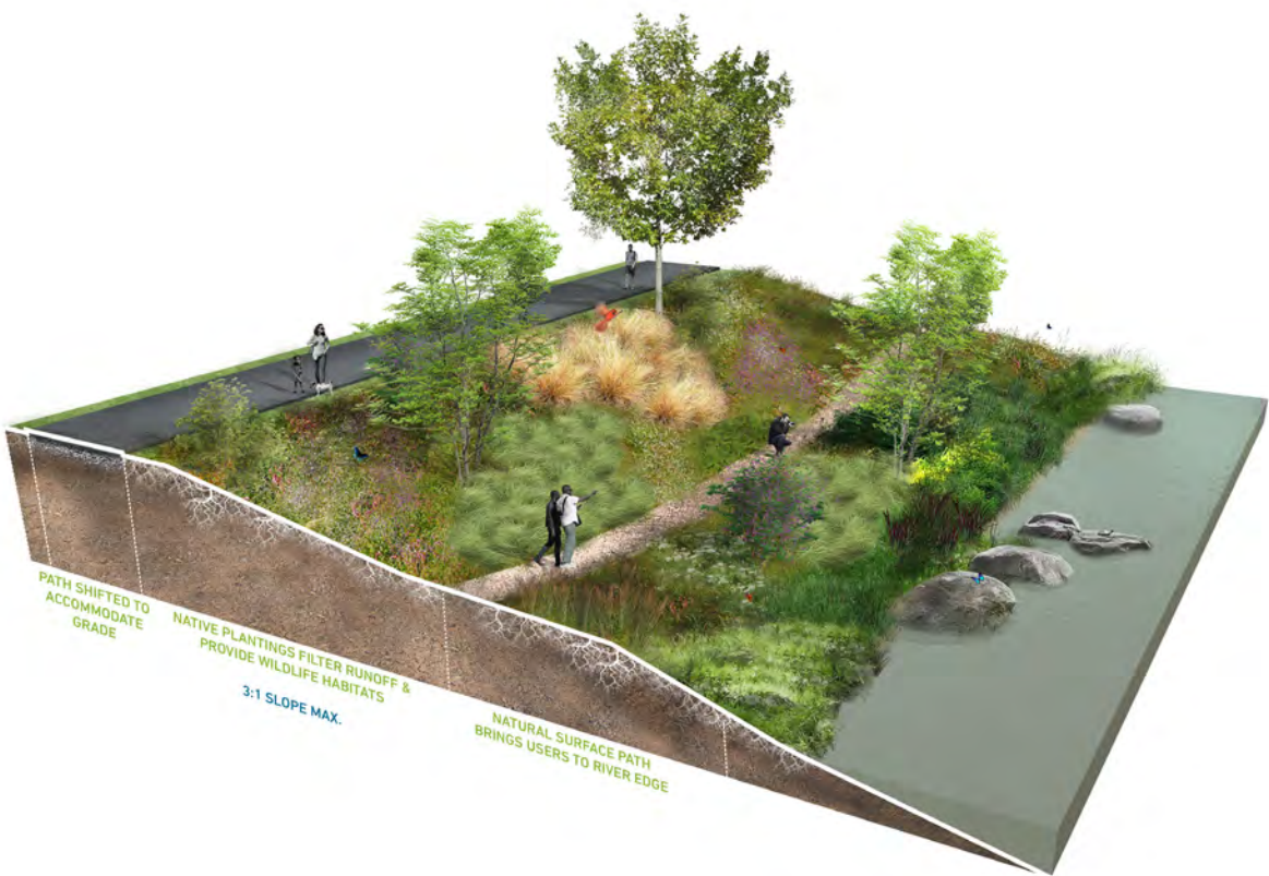
Substantial Intervention - River Benching
