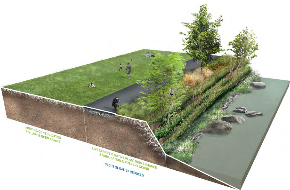
Minimal Intervention - Live Staking
